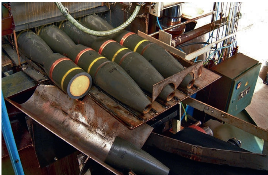
The saw-cutting of high-explosive projectiles exposes their energetic content, after which the components travel on a conveyor belt to the next station to melt out the explosives. Lübben, Germany, 2012. Source: Spreewerk Lübben GmbH
